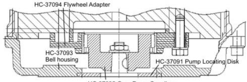
HC-37092 Gear Pump Coupling
